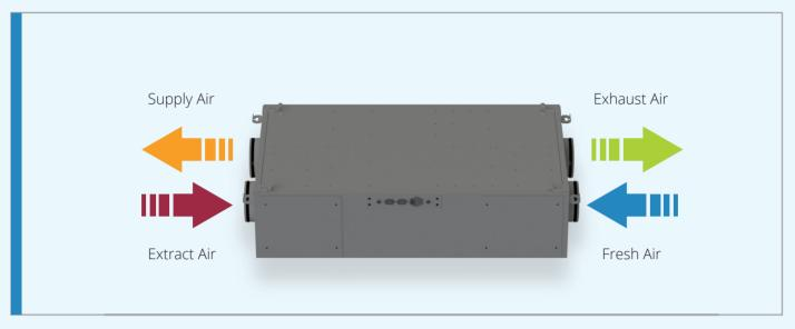
Heat recovery units are used to reduce the energy required to heat or cool the buildings. This is done by recovering the residual heat of the exhaust air and transferring it to the supply air by the means of heat exchangers. BSK BRHU Plus units use high thermal efficiency heat exchangers to transfer up to 85% of this heat, back into the ventilation system, significantly improving both the energy efficiency and the air quality of a building.
