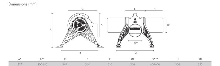
\* 'A' shown where B is 725mm. Height will change if B dimension changes. \*\* Variable to allow for adapting product height. \*\*\*Variable to adapt to differing joist widths.
