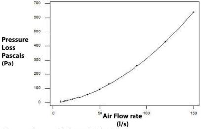
\*Pressure losses with Control Disk 10mm open
