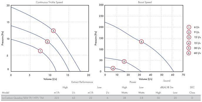
$<sup>{}^\</sup>star FID$  Performance. Tested in through the wall installation
