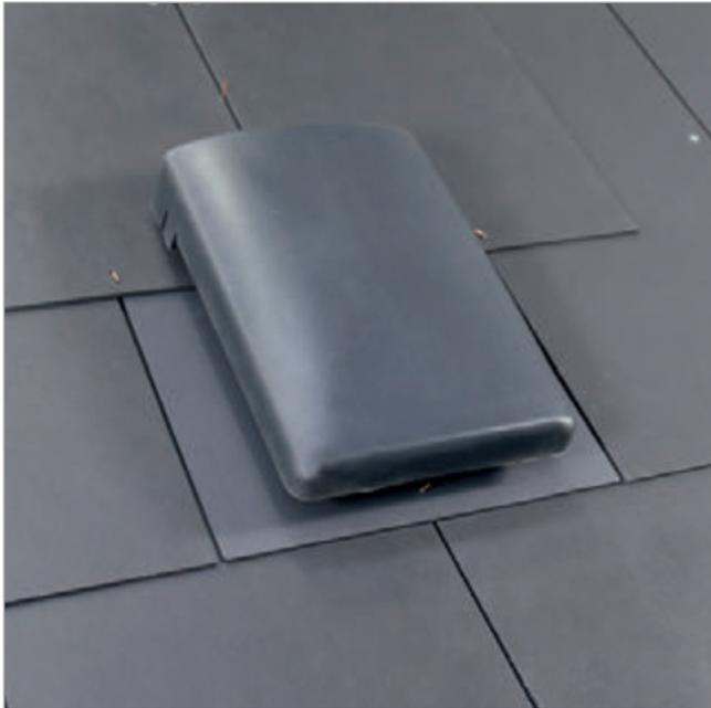
20k Slate Vent is a large capacity ventilating slate to suit 600mm x 300mm (24" x 12") and 500mm x 250mm (20" x 10") double lap slates, man-made or natural, for roofs with a pitch over 22.5°.
