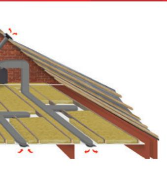
Site constraints such as shallow ceiling void spaces can be overcome with the low profile 204x60mm rectangular. While high airflow ducting requirements to combat today's apartment purge ventilation needs, can be achieved using our 220x90mm rectangular system.
