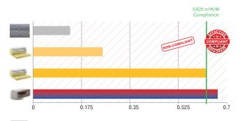
Aluminium Coated Bubble Foil 4mm Thick (1 Laver) with Thermal Conductivity 0.03 W/mK Mineral Wool 10mm Thick with Thermal Conductivity 0.04 W/mK Mineral Wool 25mm Thick with Thermal Conductivity 0.04 W/mK Verplas Self-Seal Thermal with Thermal Conductivity 0.03 W/mK
