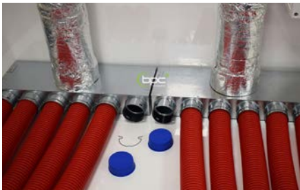
Any unused ports on the distribution box need sealed by first removing the pipe retaining clip.
